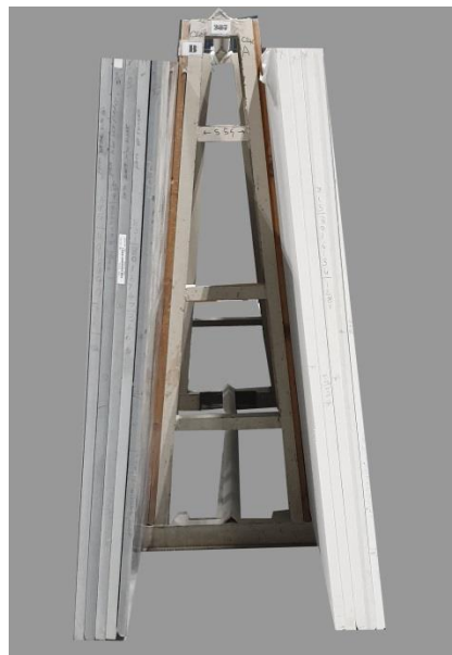
'A' Frame for Slab storage
